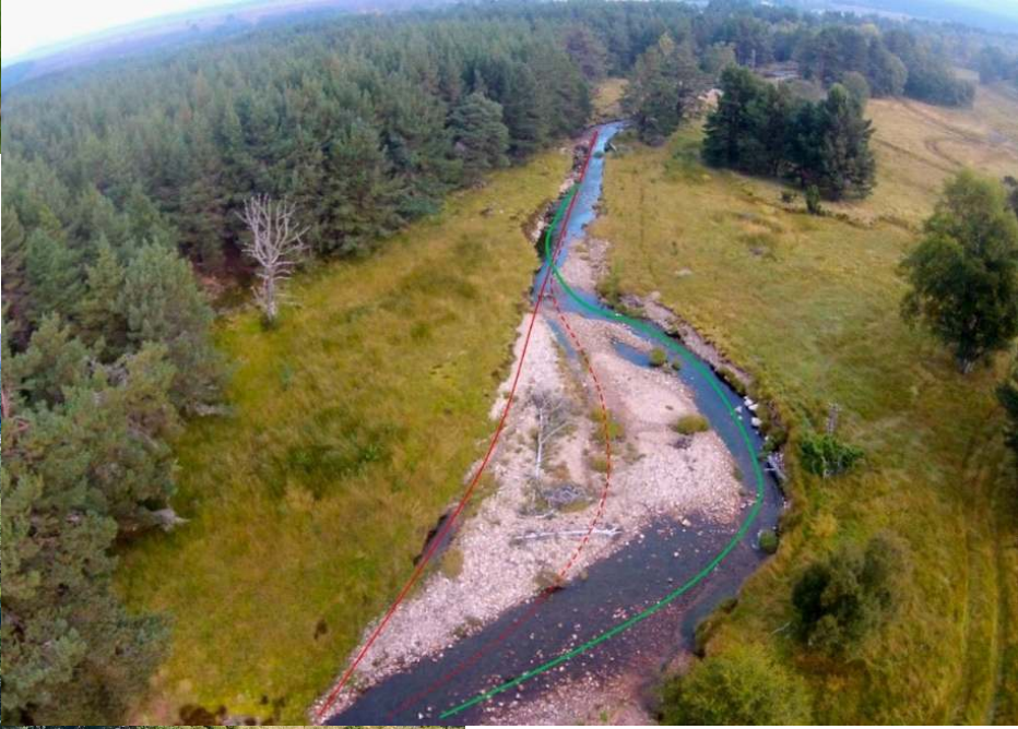
Above: The Allt Lorgy in 2016, four years after the initial restoration work and adoption of a “Stage Zero” approach having started to find its own meander.
